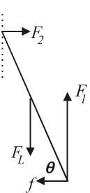
The pivot point is the base of the ladder.
