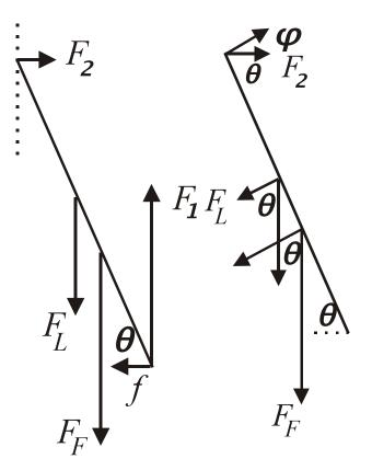
$$F_2 = \frac{500.0 \, N \cos 60.0^{\circ} \, \left(7.50 \, \text{M}\right) + 800.0 \, N \cos 60.0^{\circ} \, \left(4.00 \, \text{M}\right)}{\cos 30.0^{\circ} \, \left(15.0 \, \text{M}\right)}$$
