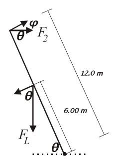
A 15 m, 500.0 N uniform ladder rests against a frictionless wall. It makes 60.0° angle with the horizontal. Find (a) the horizontal and vertical forces on the base of the ladder if an 800.0 N fire fighter is standing 4.0 m from the bottom. If the ladder is on the verge of slipping when the fire fighter is 9.0 m from the bottom of the ladder, (b) what is the coefficient of static friction on the bottom?
